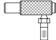
Ball Joints are usually loaded radially, however, axial pull out loads should still be considered to avoid the ball stud pulling out of its corresponding socket when fully articulated. Life expectancy is dependant on many application variables. Therefore we ask our customers to carry out their own testing once we have recommended a suitable linkage configuration.
