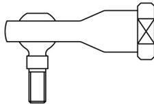
When designing a control linkage a Ball Joint with very little or no backlash is an advantage to provide a nice positive feel to the controls of the machine. Vibration is another factor. A Ball Joint fitted to the control pump of a Skidsteer will encounter a tremendous amount of vibration and could promote premature wear. When space is an issue, a Ball Joint is usually preferred over a Rod End (Sometimes known as a Rose Joint).
