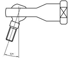
In some instances where there is minor misalignment between parts to be linked, an In-line Ball Joint will be suitable but note that these are not designed to be used under tension.
